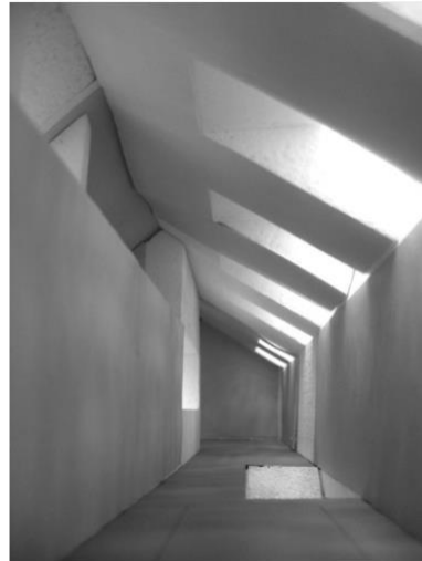
Daylight in a model under artificial sky
